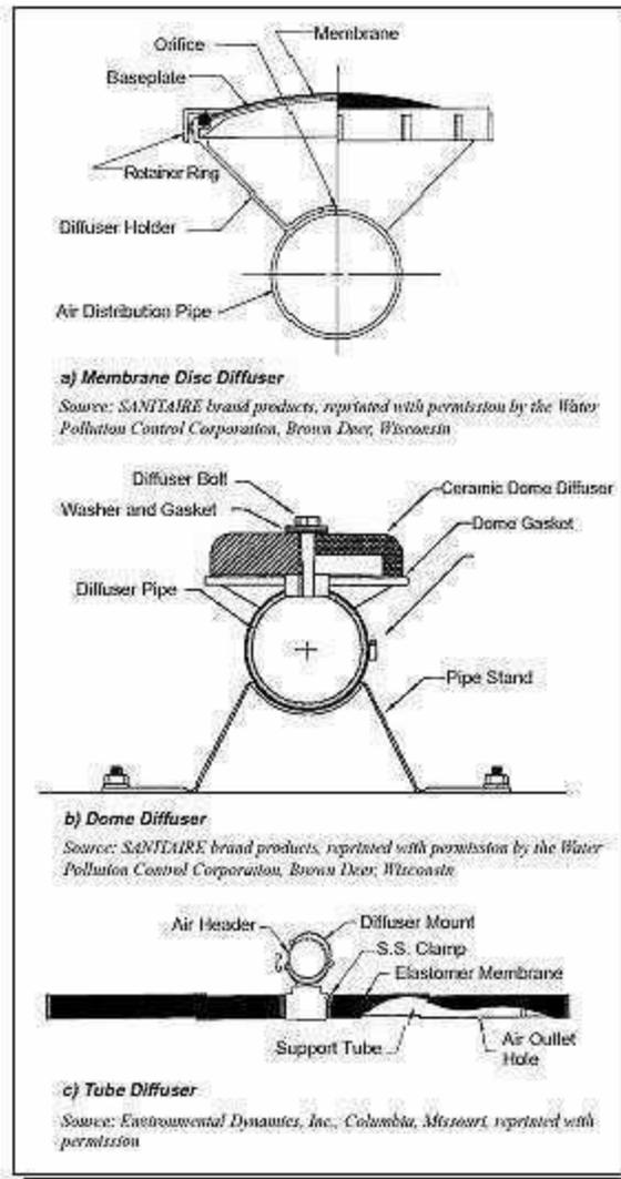
**Figure 1: Schematic of Various Fine Bubble Diffusers**
