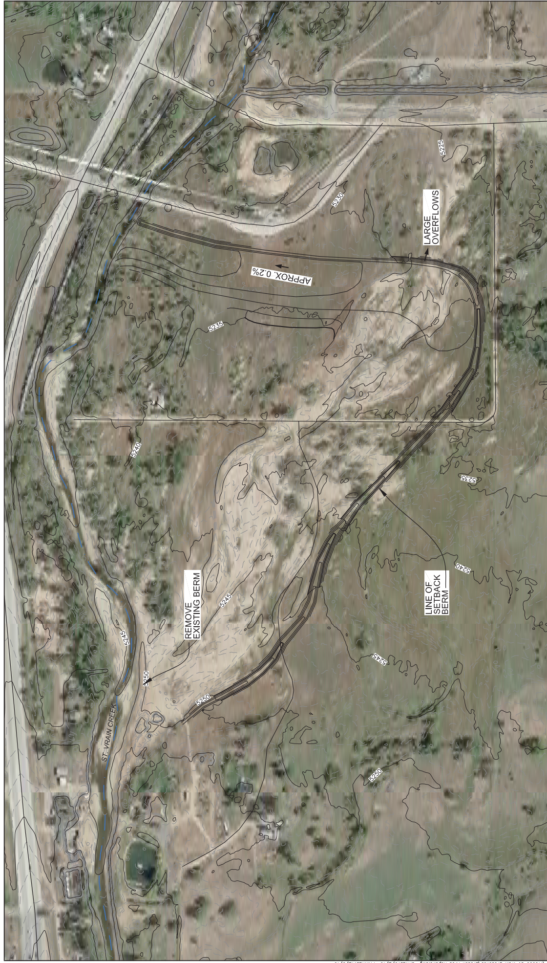
FIGURE 4-1C BREACH 1, ALTERNATIVE 3 MAXIMUM FLOODPLAIN SETBACK BERM
