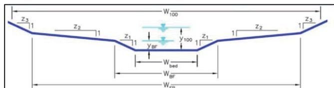
**Figure 8 Example stable channel design template**
