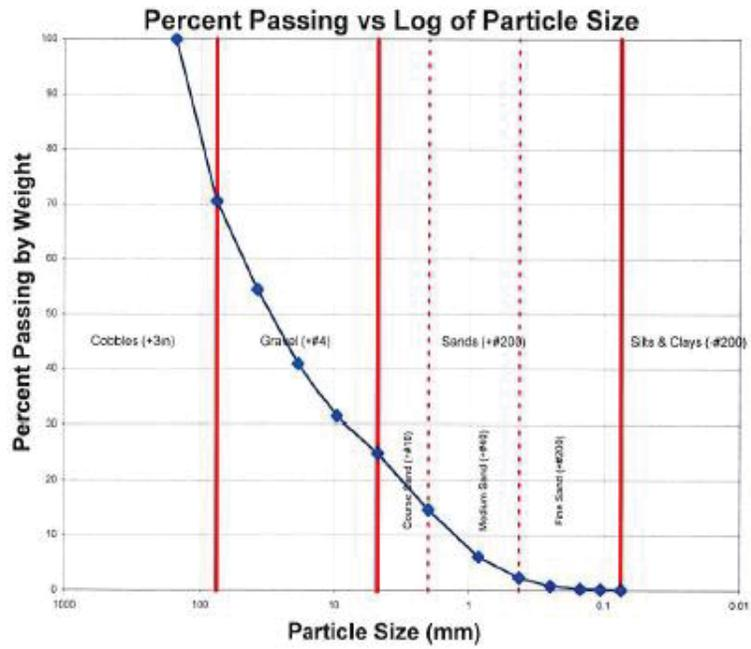
Figure 3 Channel Pavement and Sub-Pavement Material Distribution
