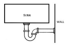
Direct waste lines connect continuously from the sink basin or fixture to the sanitary sewer.
