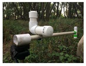
Line-point Intercept Survey Tool: periscope (for canopy cover) mounted on arm with laser (for ground cover)
