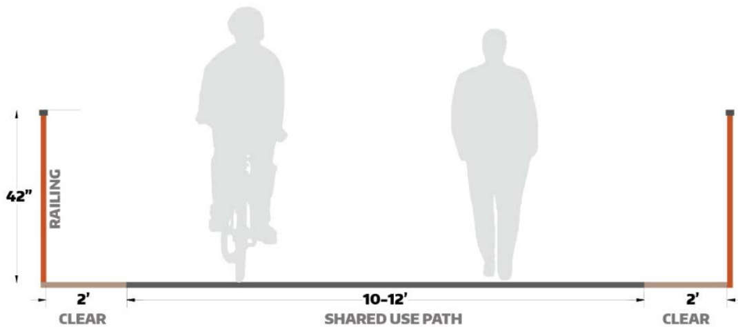
Figure 3: Typical Overpass / Bridge / Creek Crossing Configuration
