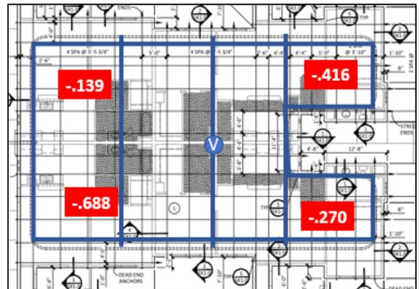
Flat Mat Layout and With Negative Pressures Developed with Temporary Radon Fan (IN W.C.)
